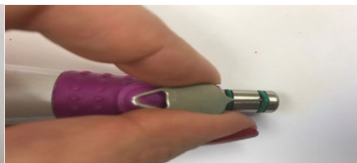
Replacing O-rings on the Outer Sheath
