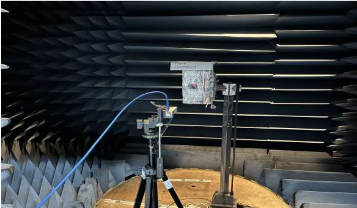
Photograph: Measurement set-up 18-40GHz, EUT standing
