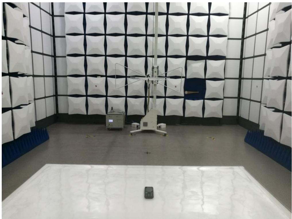
RADIATED EMISSION ABOVE 1G TEST SETUP
