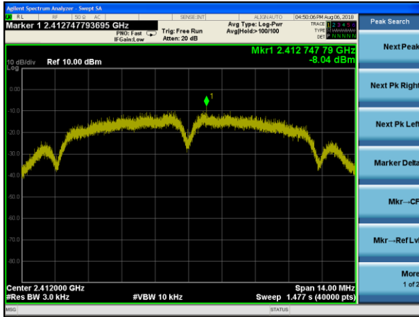
(802.11b) PSD plot on channel 6
