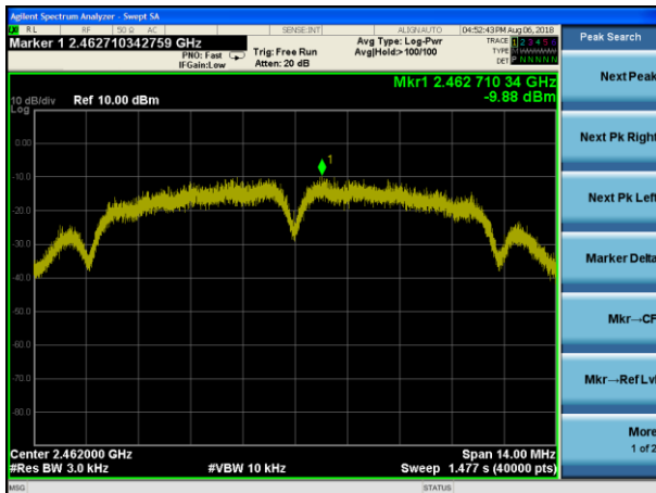
(802.11b) PSD plot on channel 11
