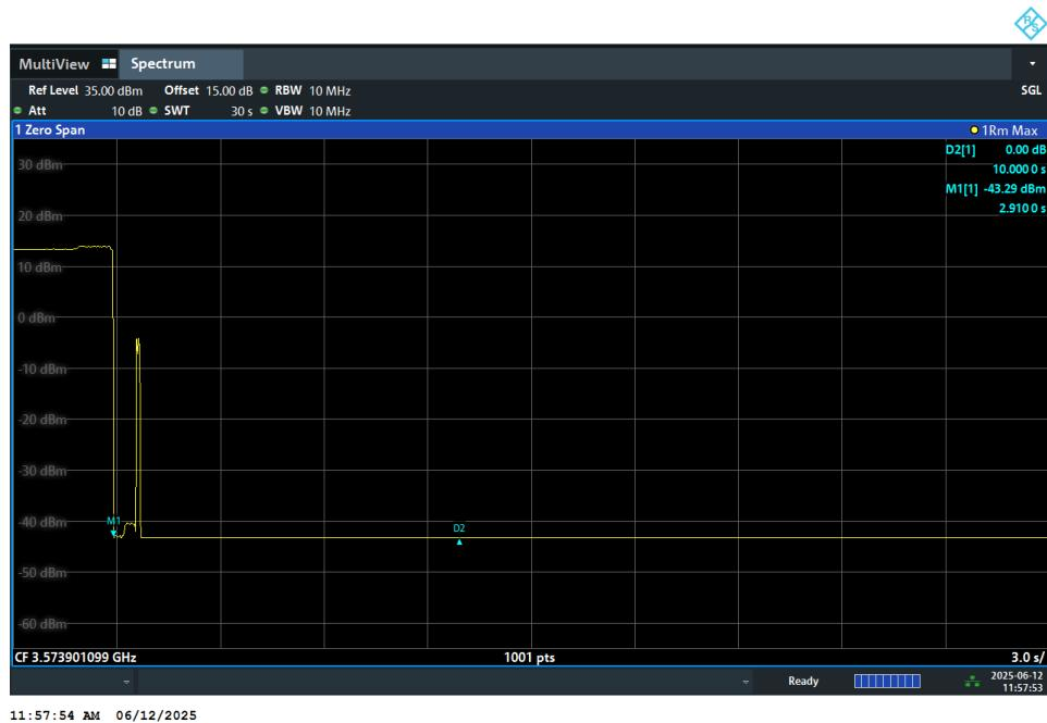
**[Step 5] Configure SAS granted CBSD to operate at frequency 3650-3690 MHz & power level 30 dBm/MHz**
