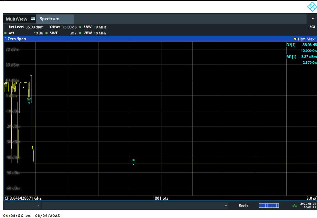
**[Step 5] Configure SAS granted CBSD to operate at frequency 3600-3700 MHz & power level 30 dBm/MHz**
