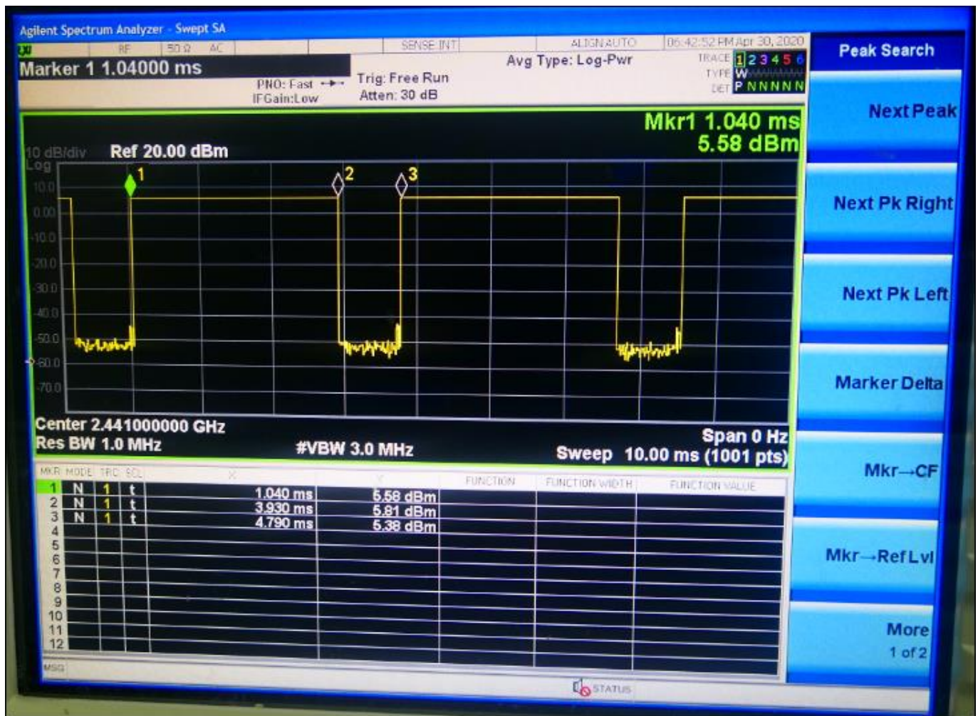
Time-domain plot for Bluetooth transmission signal
