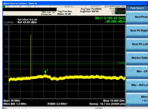
Conducted Emission Transmitting Mode CH 661
