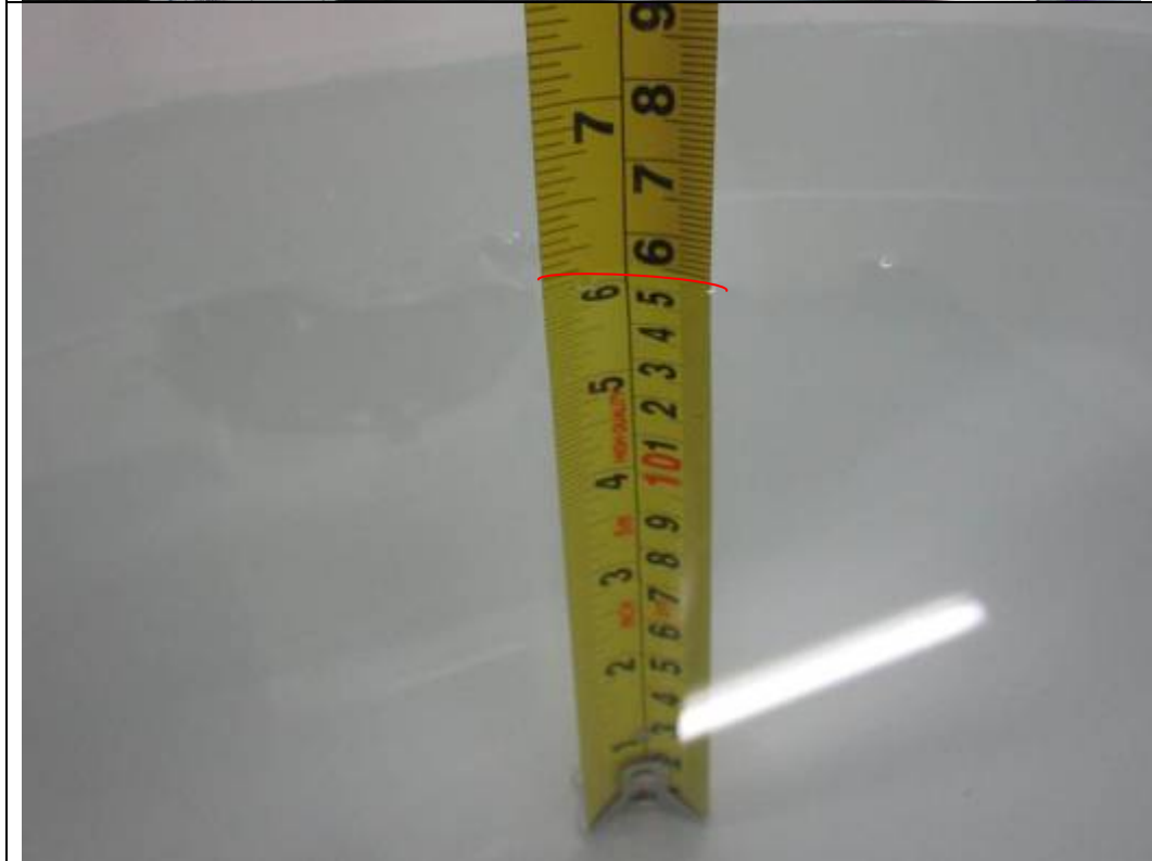
Liquid depth \geq 15cm
