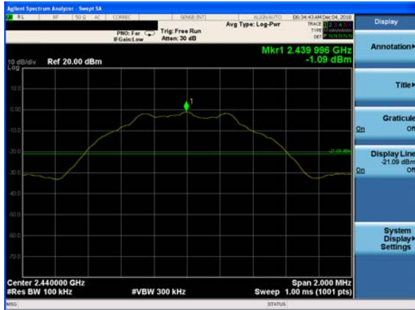
GFSK on channel 19
