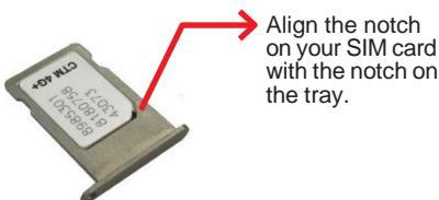
4. Place the device on a flat surface with the panel side facing down. Insert the tray into the device completely and in the same orientation that you removed it. The tray also fits only one way.
