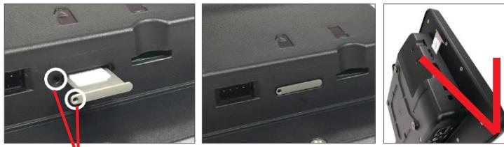
Make sure to align the hole on the tray with the hole in the device.
