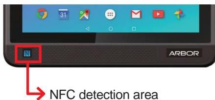
To test the NFC function, you can use the provided **NFC SmartCard Info** App to test the NFC.
