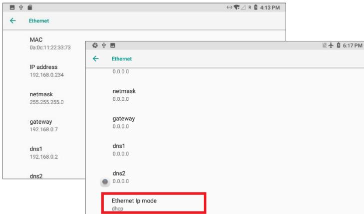
2. Tap **Ethernet IP mode** and select a IP mode according to your network environment.
