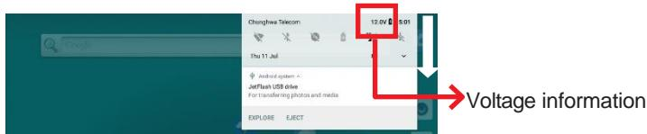
You can also configure the IOT-800N to show voltage information in the status bar. To do so, tap **Settings** | **Battery** and turn on the **Battery Voltage** option.
