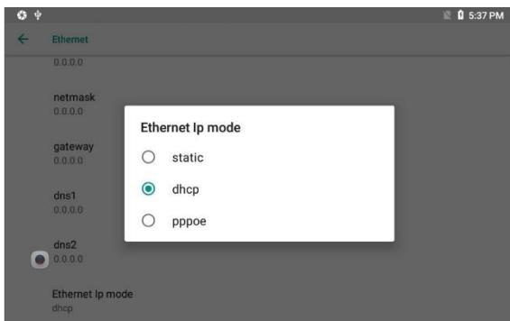
To use a static IP address, tab **static** and then configure the required settings. When you're done with the settings, tap **CONNECT**.
