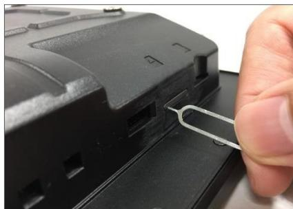
3. After ejecting the SIM card tray, place your SIM card into the tray. Note that there is a notch in one corner to ensure the SIM card is placed correctly.
