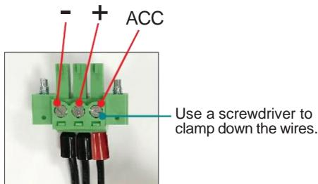
2. Plug the terminal block into the power connector and then tighten the screws to secure the terminal block in place.
