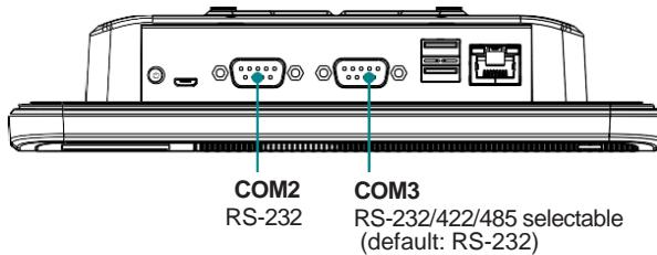
To configure the mode of COM3 or the settings like baud rate of COM2 & COM3, you have to use the **SerialPort API** as described below:
