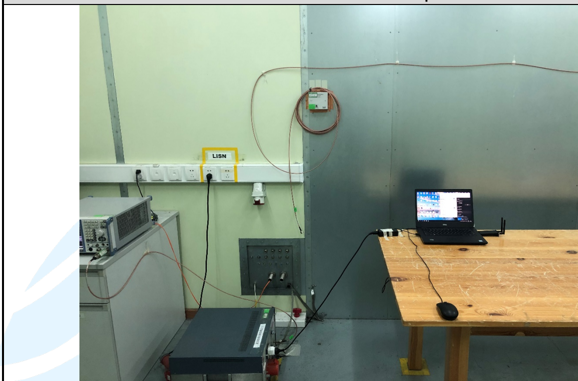
Conducted Emission Test Setup
