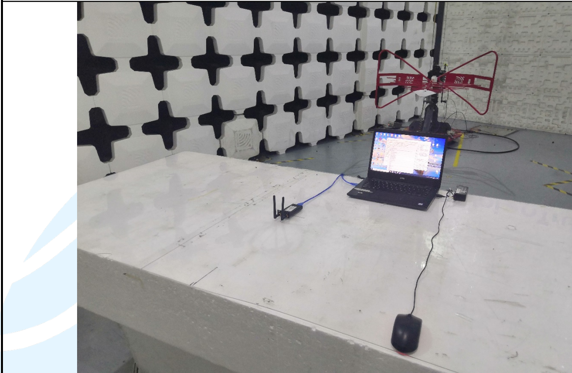
Radiated emission Test Setup (30 MHz~1 GHz)
