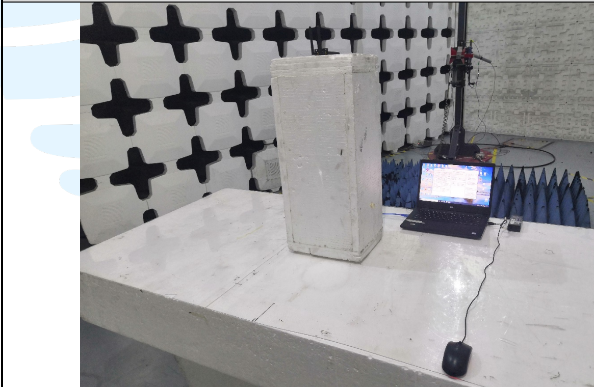
Radiated emission Test Setup (Above 1 GHz)
