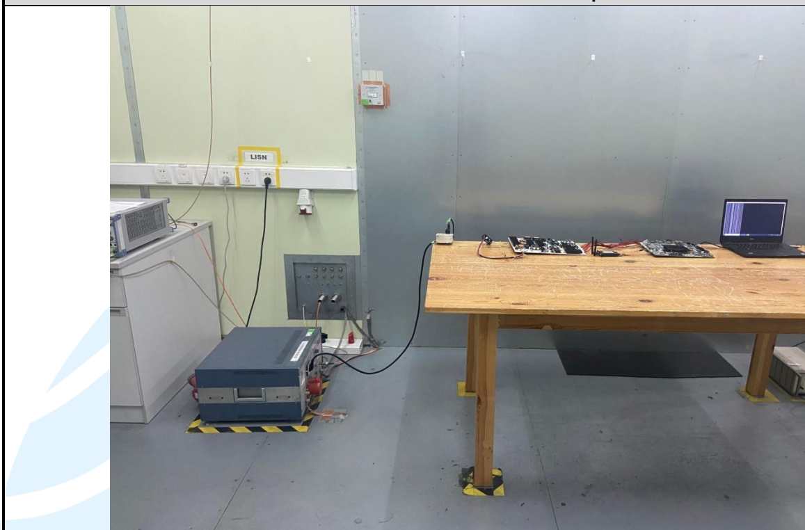
Conducted Emission Test Setup
