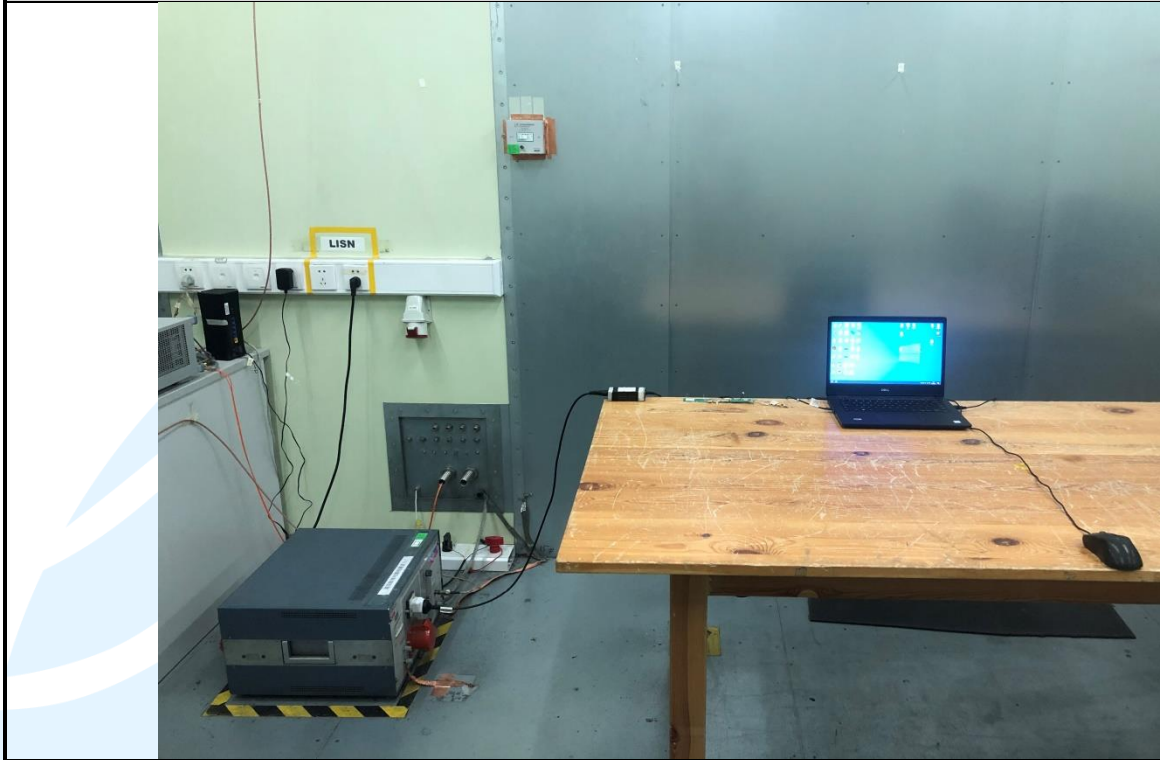
Conducted Emission Test Setup
