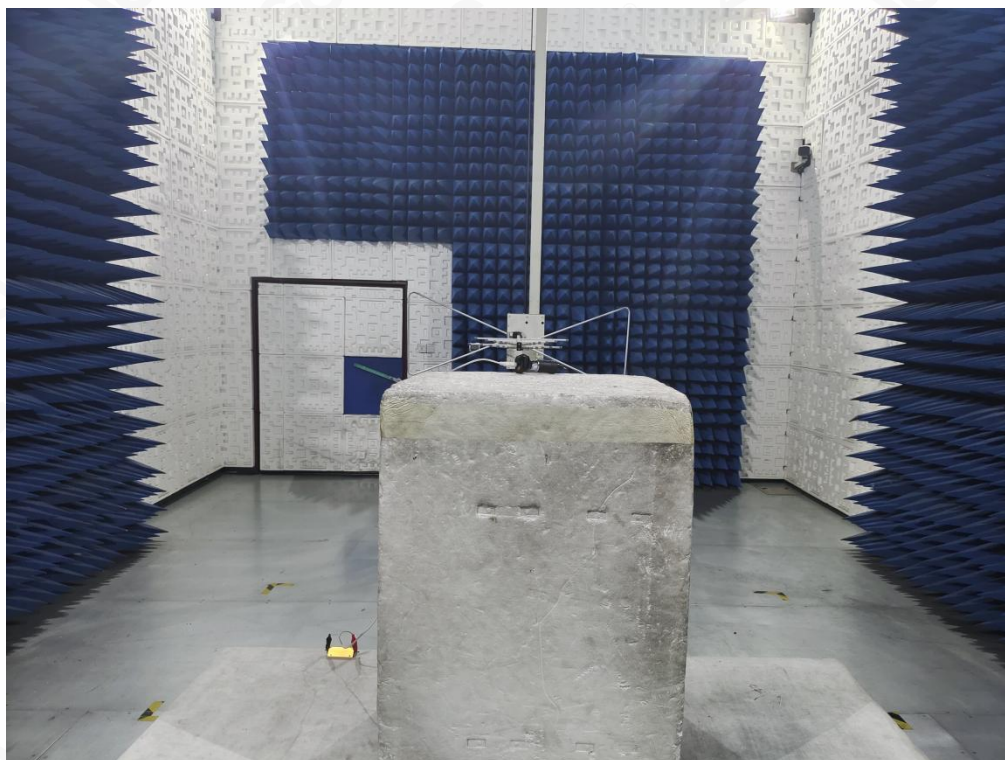
RADIATED EMISSION TEST SETUP ABOVE 1G
