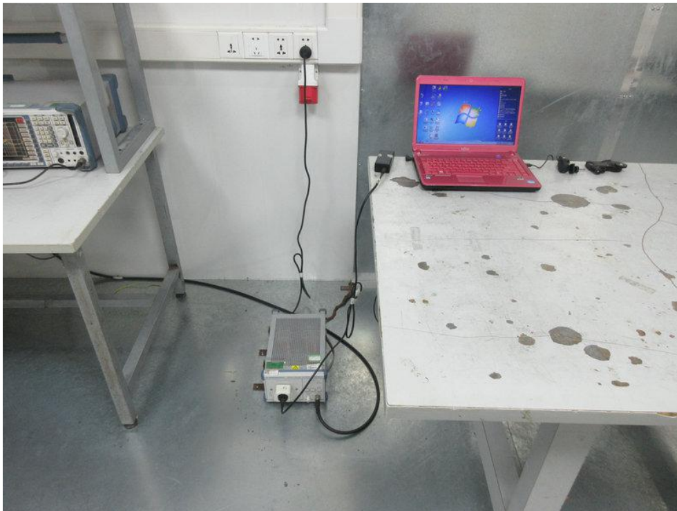
Photo of Power Line Conducted Emission Test
