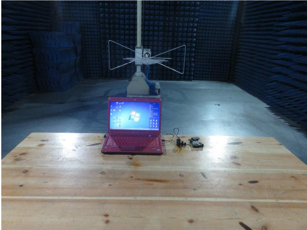
Photo of Radiation Emission Test
