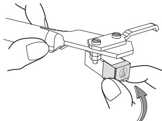
3. Make sure there is no gap between the head shell and the cartridge.
