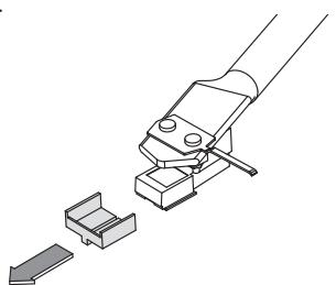
**NOTE:** Applying a downward force may cause the stylus to come off the body. Only low volume is output if the stylus has come off, or is about to come off, so refer to **"Replacing the stylus"** to reattach the stylus correctly.
