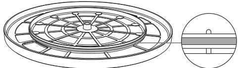
2. Set the platter on the spindle. Make sure the platter is fully seated on the spindle.
