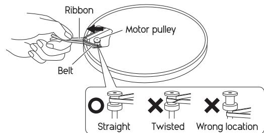
4. Finally, remove the red ribbon from the belt.
