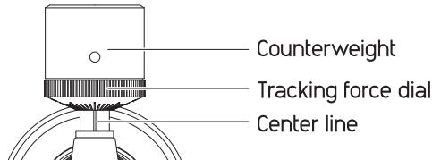
1. Gently push and turn the counterweight onto the rear of the tonearm (with the dial facing toward the front of the turntable).
