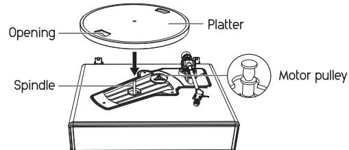
3. Place the belt on the motor pulley. Align one of the platter openings with the motor pulley, and while pulling both ends of the red ribbon that comes attached to the belt, place the belt on the motor pulley, as per the diagram. When doing this, be careful not to twist the belt.
