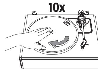
2. This step is for resetting the auto mechanism, getting rid of any twists in the belt and making sure the belt rides smoothly along the drive rim on the underside of the platter.
