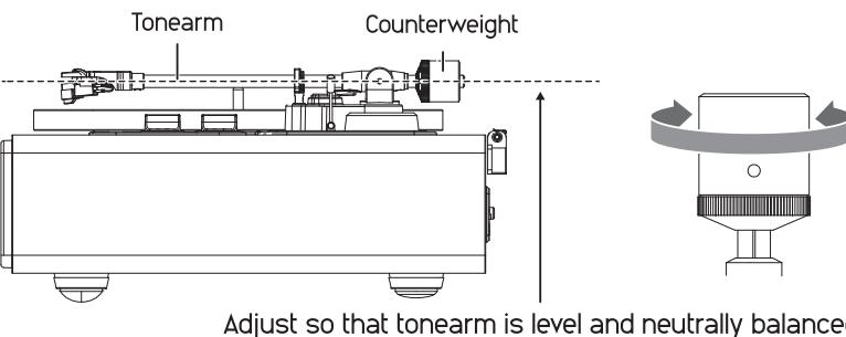
6. Once the tonearm is correctly balanced, return the tonearm to its rest and secure it in place with the clip. Hold the back of the counterweight to avoid moving its position, gently rotate the tracking force dial until the zero is in line with black center line on the rear of the tonearm. Check to make sure the tonearm is still neutrally balanced.
