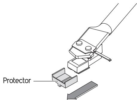
**NOTE:** Applying a downward force may cause the stylus to come off the body. Only low volume is output if the stylus has come off, or is about to come off, so refer to "Replacing the stylus" to reattach the stylus correctly.
