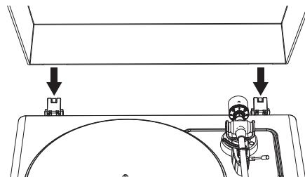
**NOTE:** It is recommended to install the lid at last to make it easier during setup and calibration.
