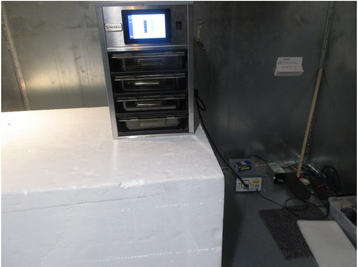
Figure 5: Power Line Conducted Emissions – Front View
