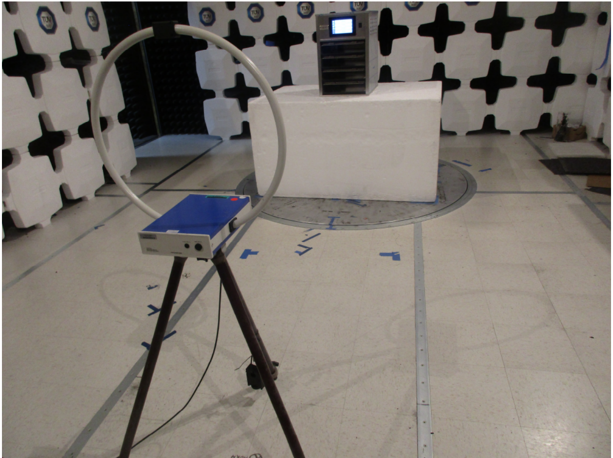
Figure 1: Radiated Emissions – Front View – below 30 MHz
