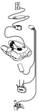
Before charging the drone make sure that the drone is turned off. Connect the power supply to the charger and connect the power supply to the wall socket. Make sure that the charging selector switch on the bottom is set to drone charging. See page 7.
