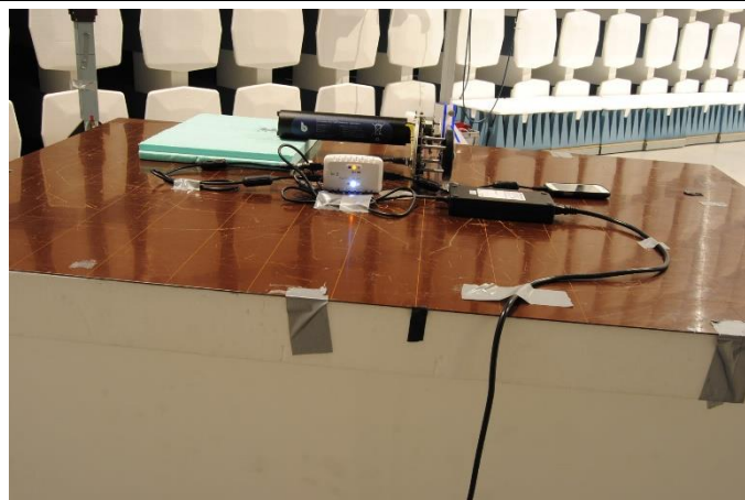
Test set-up for EMC emissions measurements
