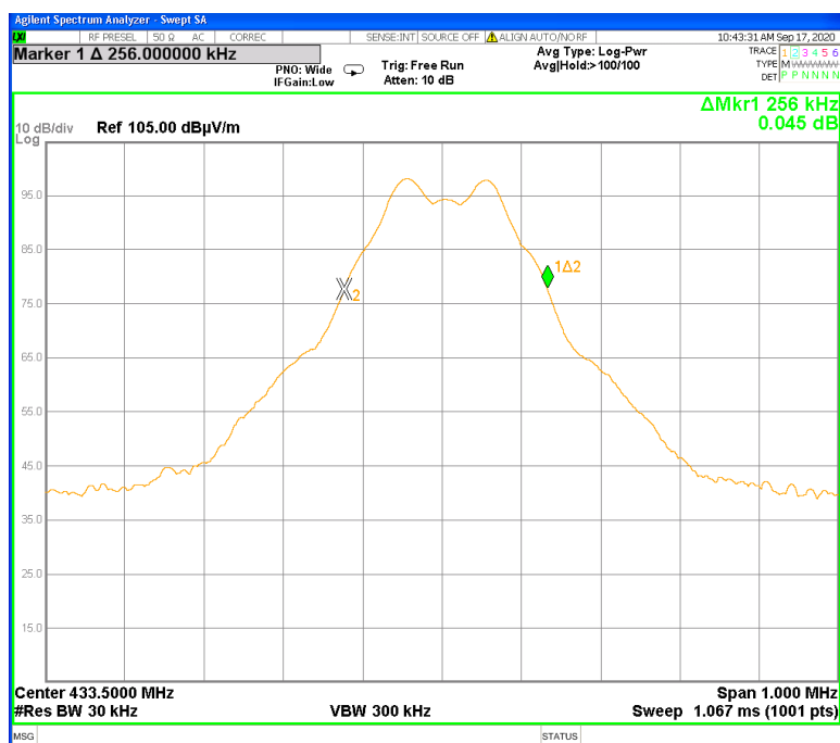
Plot # 12. Occupied bandwidth test result
