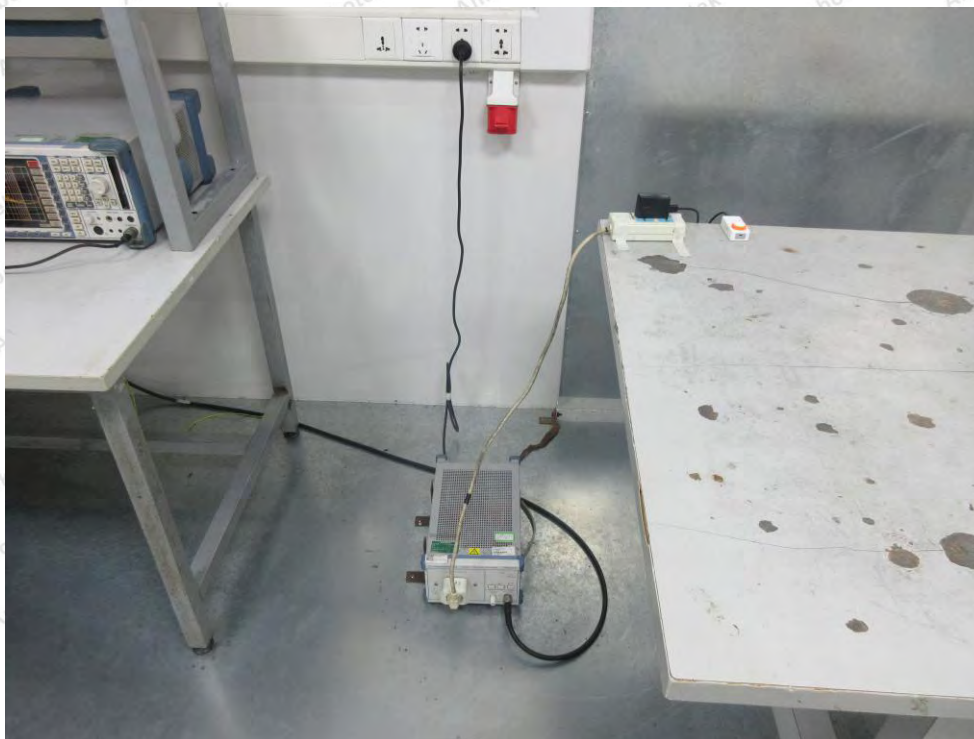
Photo of Power Line Conducted Emission Test
