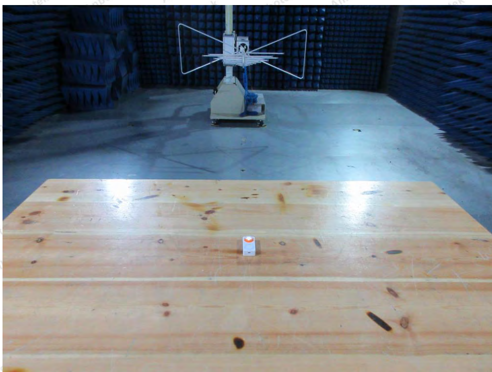
Photo of Radiation Emission Test
