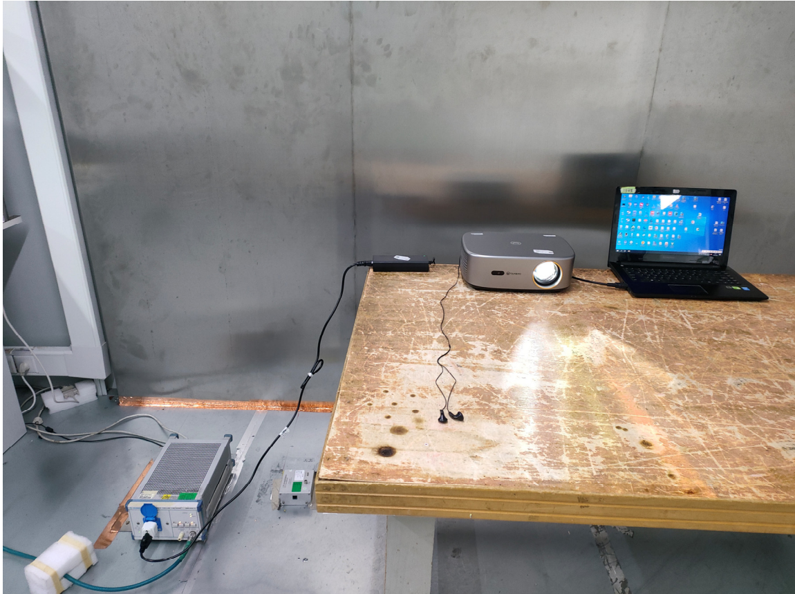
Conducted Emissions - Side View
