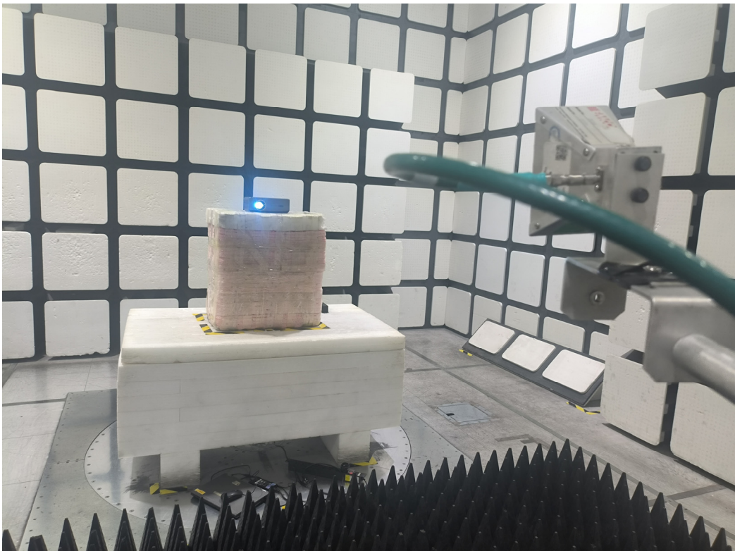
Radiated Emissions View (18-25 GHz)
