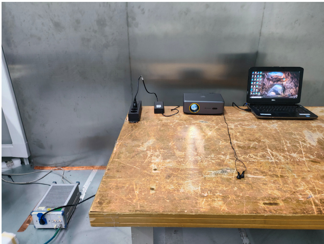
Conducted Emissions - Front View
