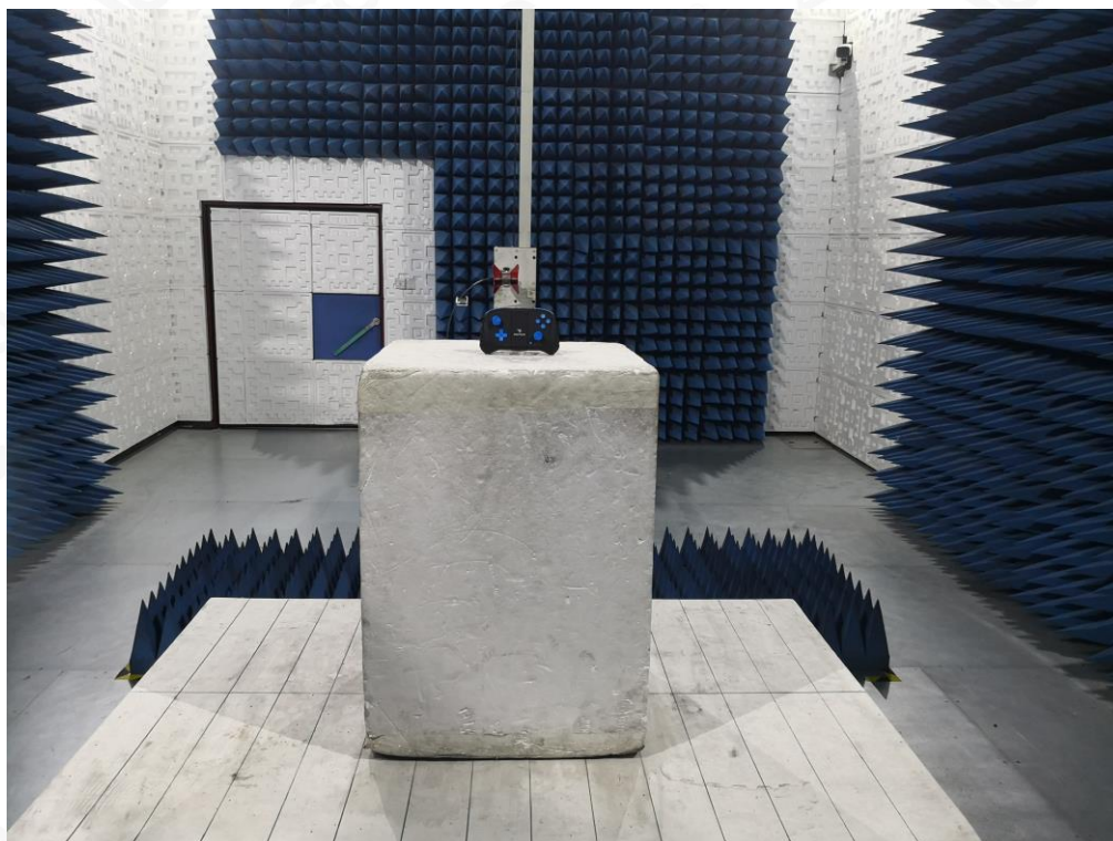
FCC RADIATED EMISSION TEST SETUP ABOVE 1GHZ
