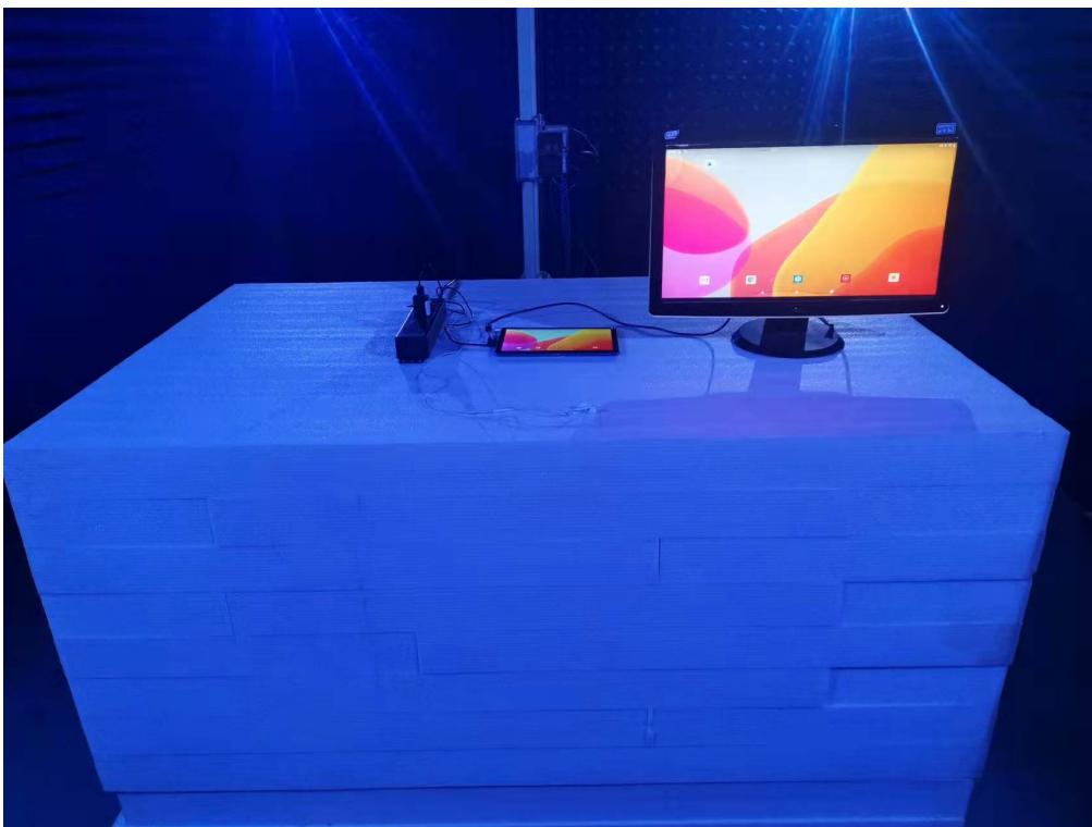
Photo of Radiated Emission Measurement (Above 1G)
