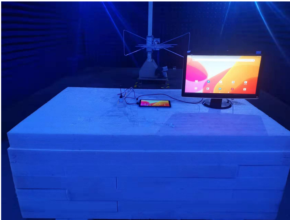
Photo of Radiated Emission Measurement (Above 1G)
