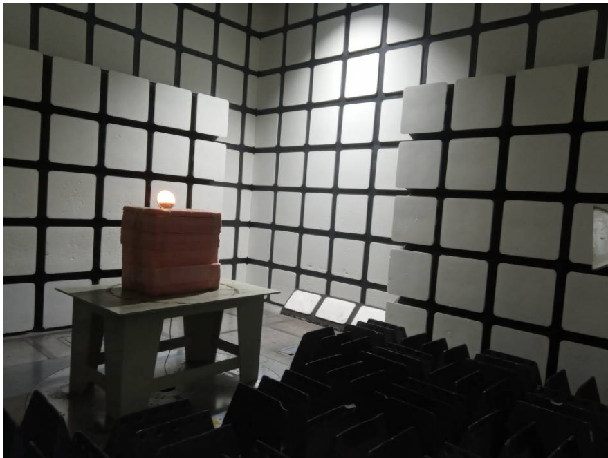
Radiated Emissions View (Above 1 GHz)
