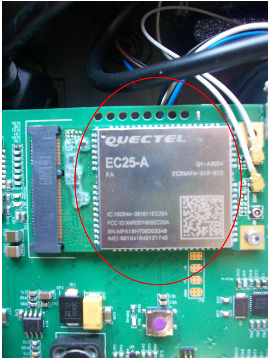
Figure 5. Closeup of Co-located Pre-Certified Module
