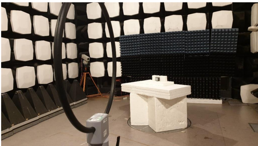
Photo 5. Radiated emission test setup in SAC. 9 kHz – 30 MHz.
