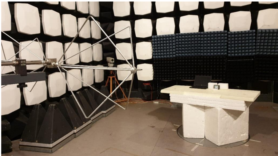
Photo 7. Radiated emission test setup in SAC. 30 - 200 MHz.
