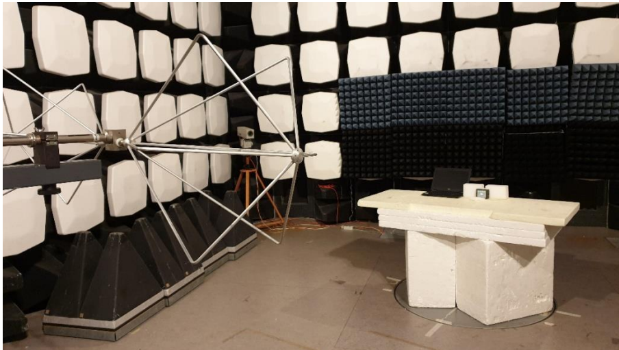
Photo 7. Radiated emission test setup in SAC. 30 - 200 MHz.
