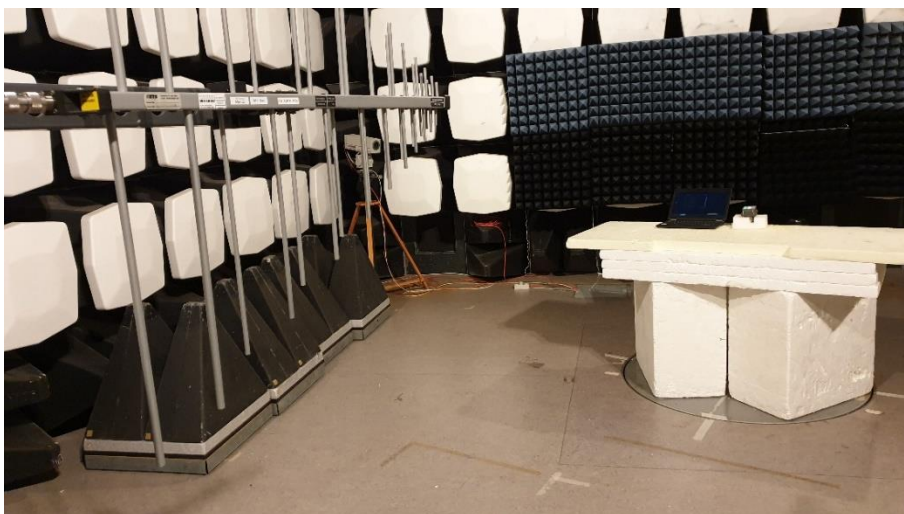
Photo 8. Radiated emission test setup in SAC. 200 - 1000 MHz.
