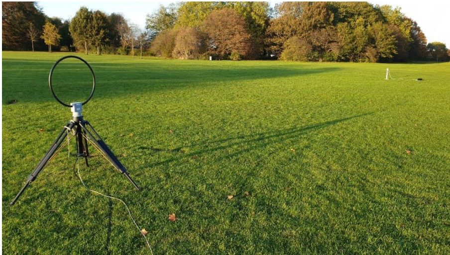
Photo 6. Radiated emission test setup at OATS. 9 kHz – 30 MHz
