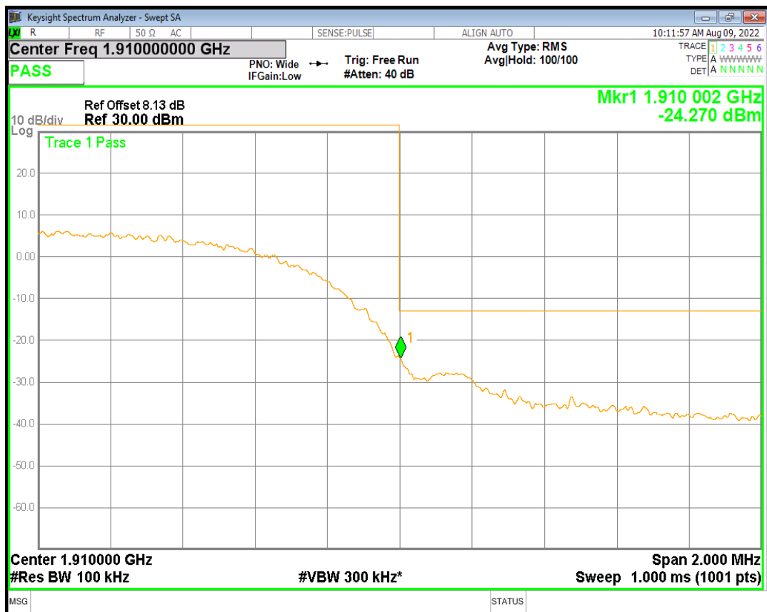
HSDPA Band5 Subtest1 Channel=4132
