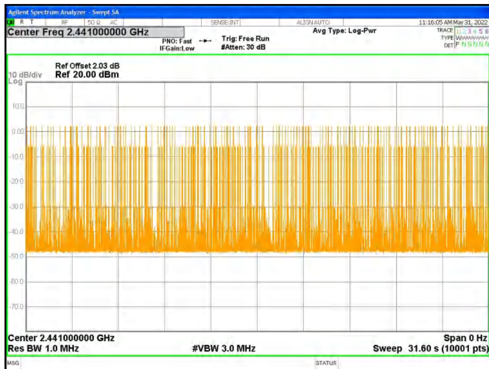
Dwell NVNT 1-DH5 2441MHz Ant1 One Burst
