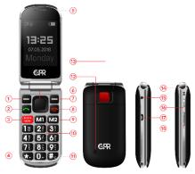
Left menu key / Main menu key 2 Dialling / History Calls 3 Block nuisance numbers 4 \* Key, Press this button on the idle screen to enter the following symbols : \* /+ /P W. 5 Receiver 6 Navi key: Key up: On the idle screen this button takes you to the Messages menu. Kev down: On the idle screen this button
