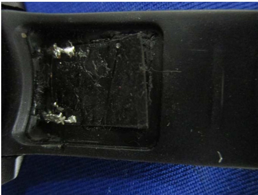
EUT – BT&WIFI&GPS Antenna View
