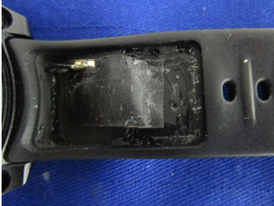
EUT – GSM&WCDMA Antenna View
