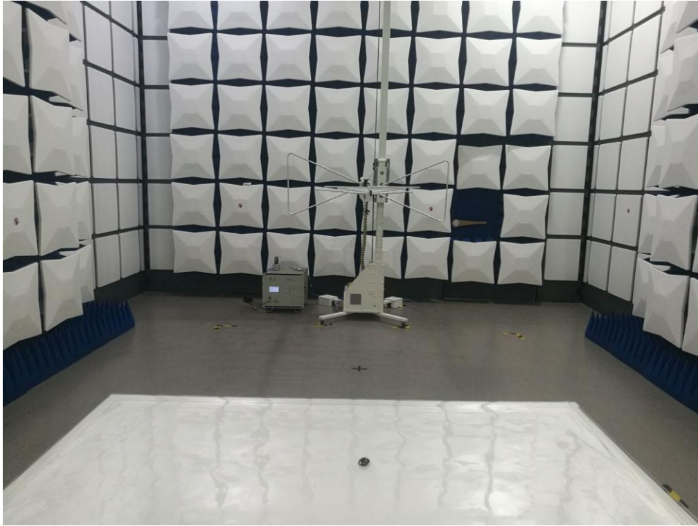
FCC RADIATED EMISSION TEST SETUP
