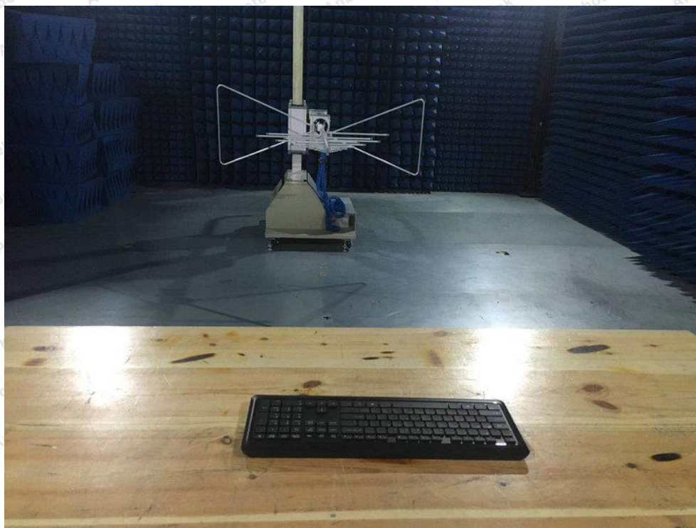
Photo of Radiation Emission Test
