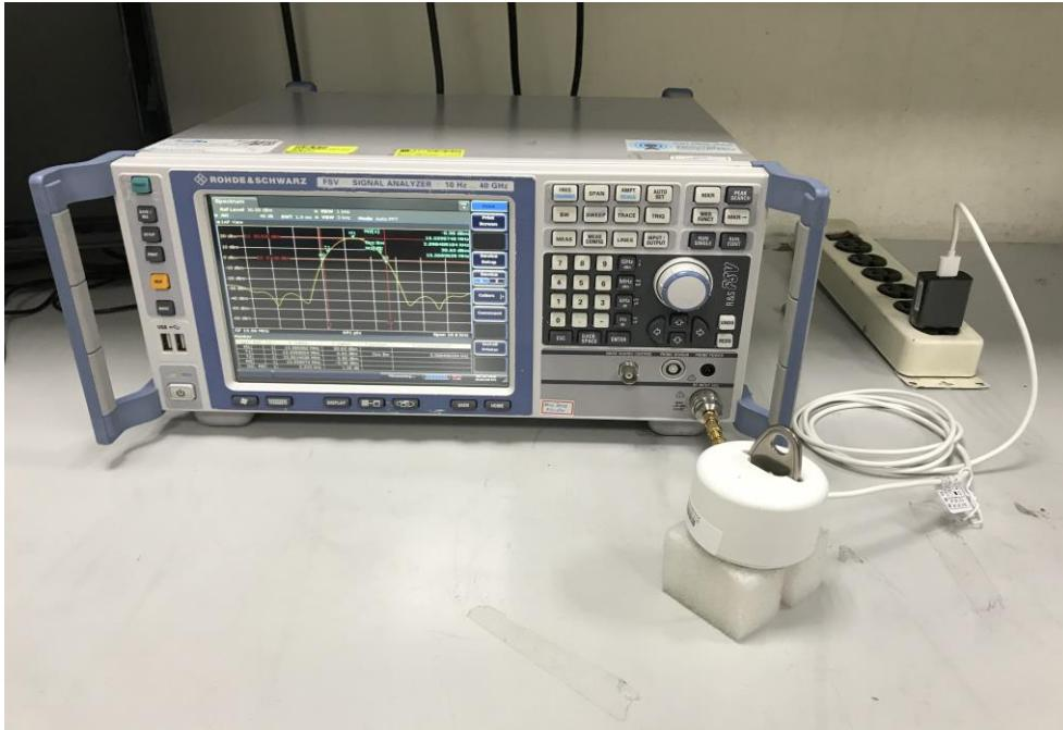
**Radiated Emission Set up Photos****9kHz ~ 30MHz**
