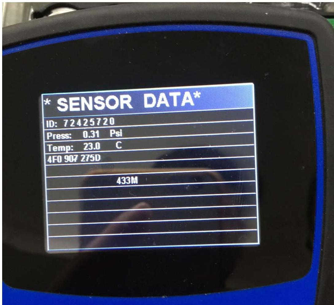
Remark:When you are programming the sensor,the sensor must be close to the programming tool.
