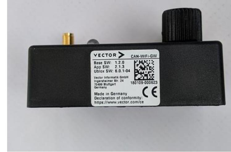
Please find below the proposed label for the component. We testify that the FCC ID is not on the module since the module will be destroyed if attempted to open as its permanently encased so as to meet the requirement as specified in the rule part.
