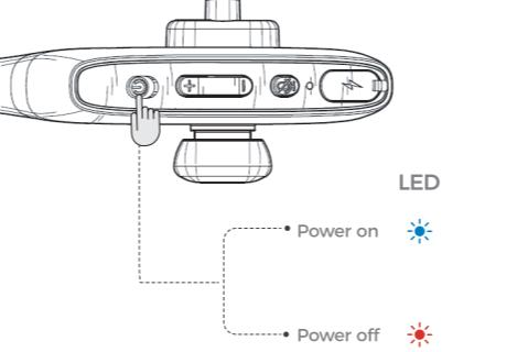
1. Enable pairing mode: Hold the multi-function button for 5s after power on.
