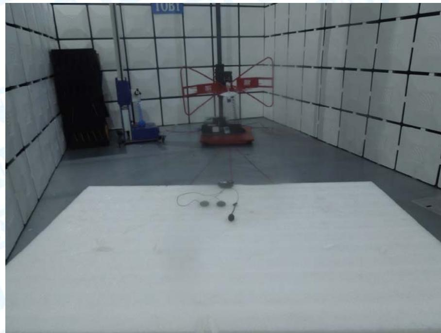
**Photo of Setup for Conducted Emission**
