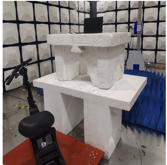
Photograph 3: Set-up photo for Radiated Spurious Emission, up 1GHz
