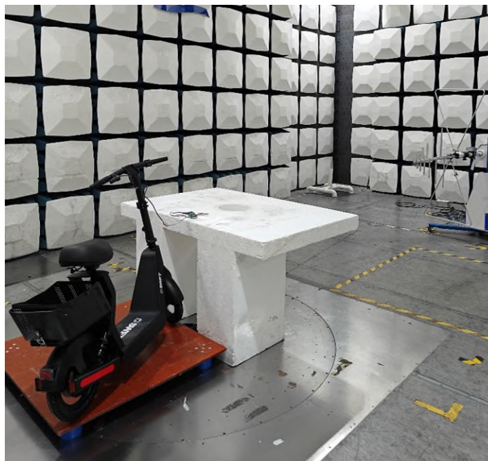
Photograph 2: Set-up photo for Radiated Spurious Emission, below 1GHz
