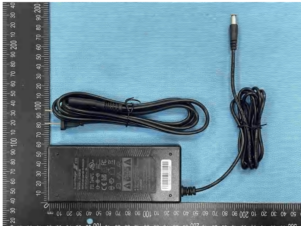
Figure 28: External adaptor view, type JY-420150
