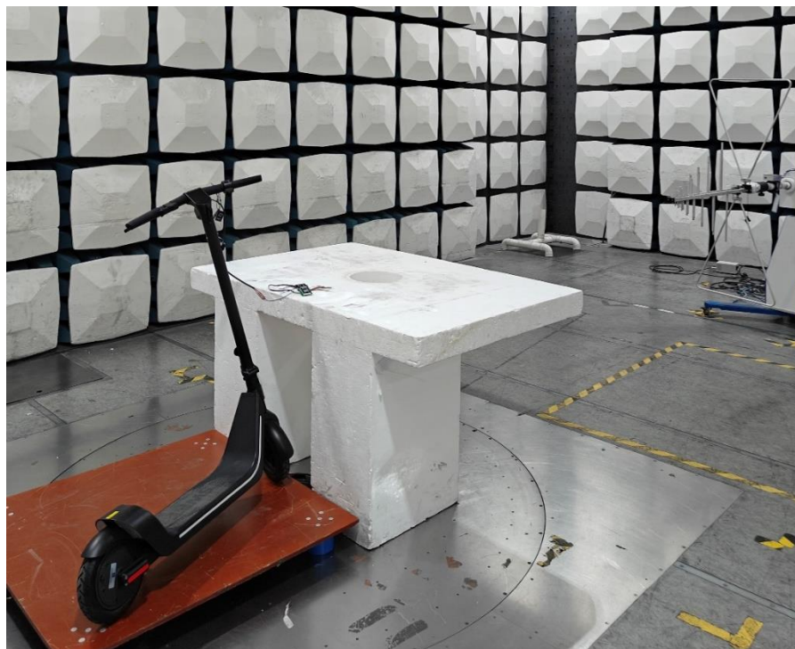
Photograph 2: Set-up photo for Radiated Spurious Emission, Below 1GHz
