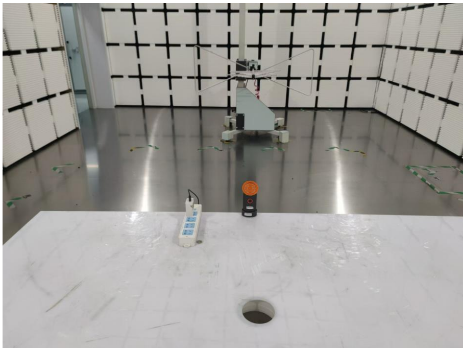
Photograph 2: Set-up photo for Radiated Emission, 30MHz - 1GHz
