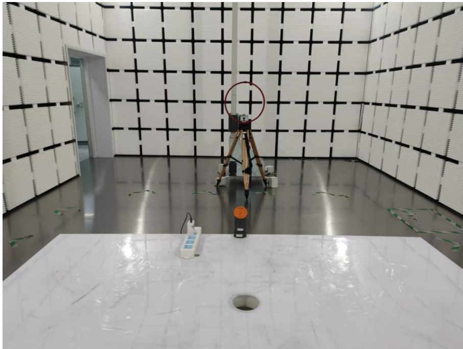
Photograph 1: Set-up photo for Radiated Emission, 9KHz - 30MHz
