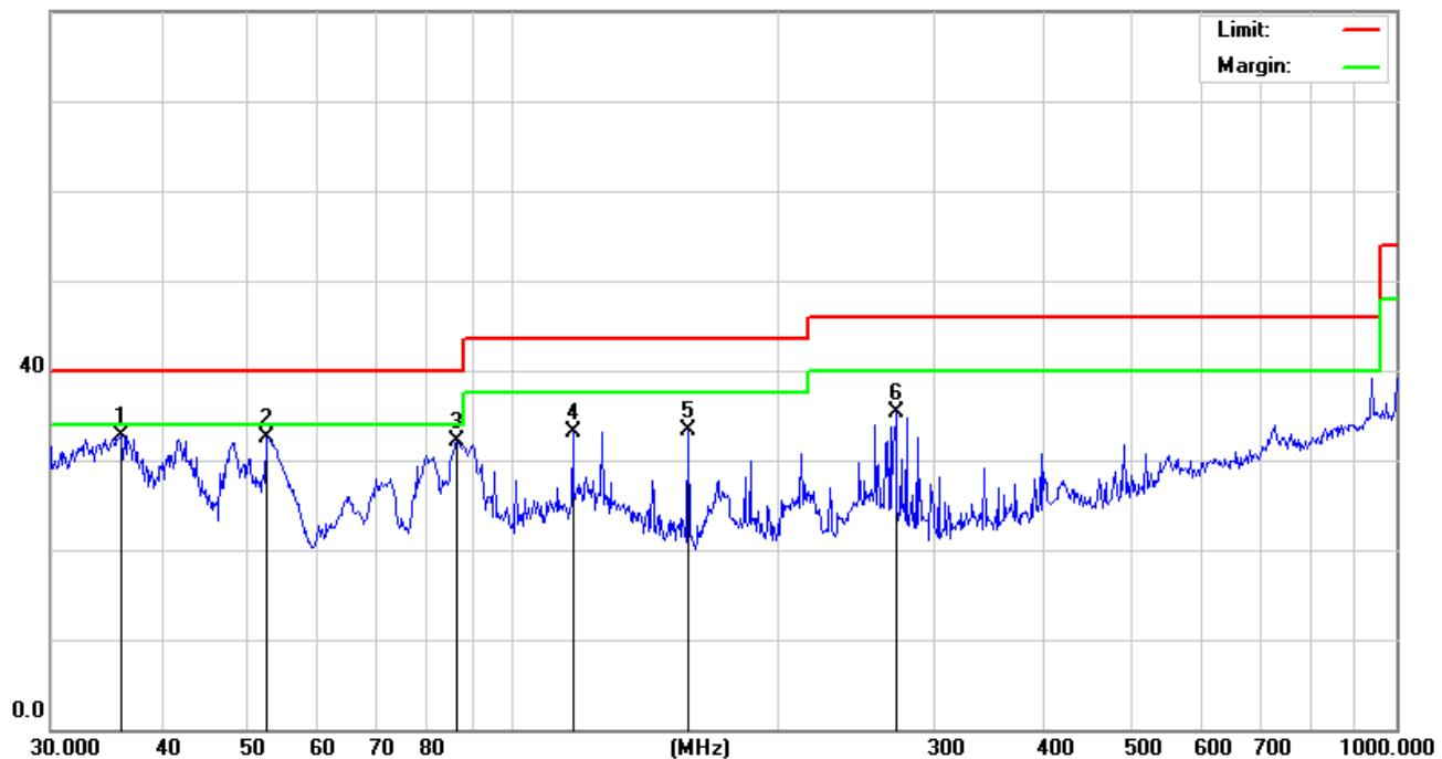
Remark: Transd = Cable lose + Antenna factor - Pre-amplifier; Margin = Limit – Level
