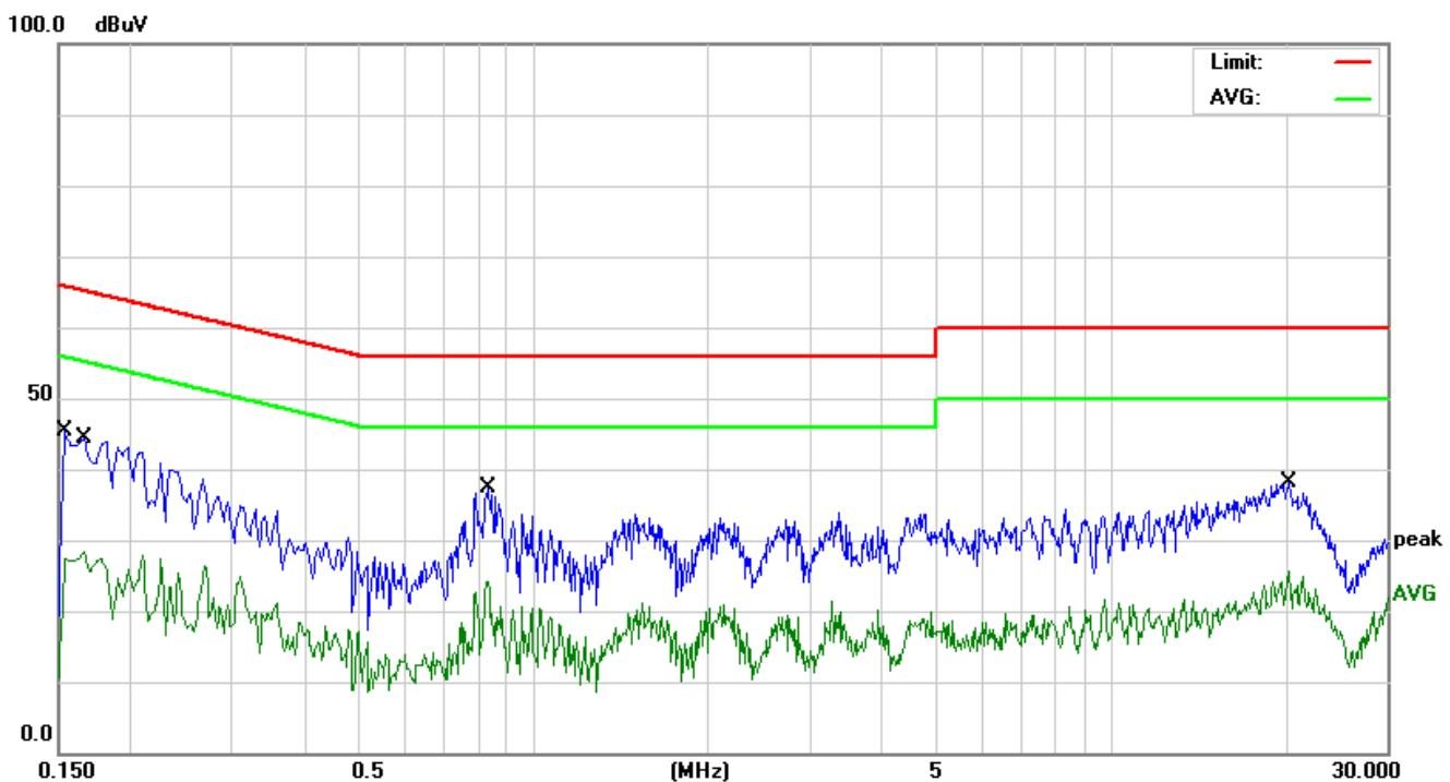
Remark: Transd = Cable lose + Antenna factor - Pre-amplifier; Margin = Limit – Level
