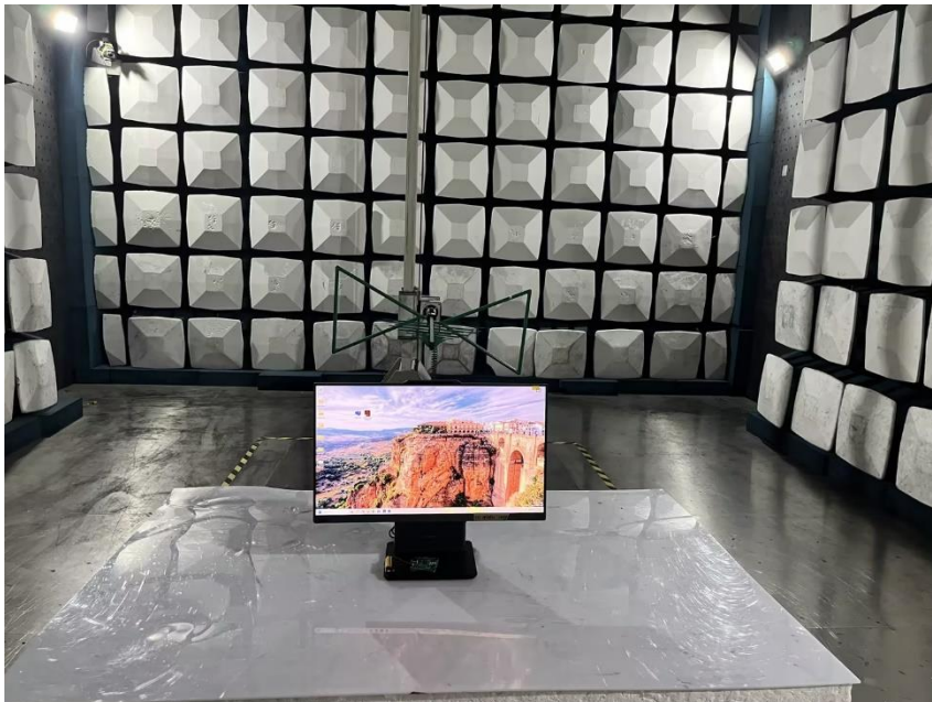
Radiated Test (30MHz-1GHz)
