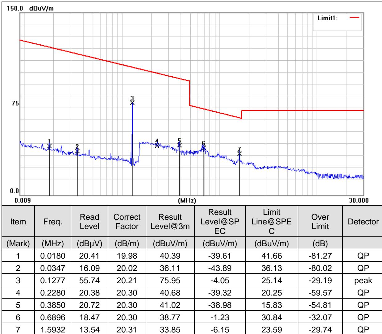
Remark: Result Level= Read Level + Antenna Factor + Cable Loss
