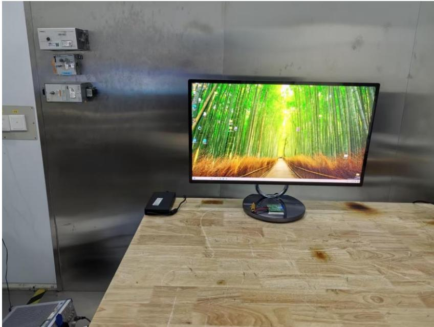
Radiated Test Below 30MHz
