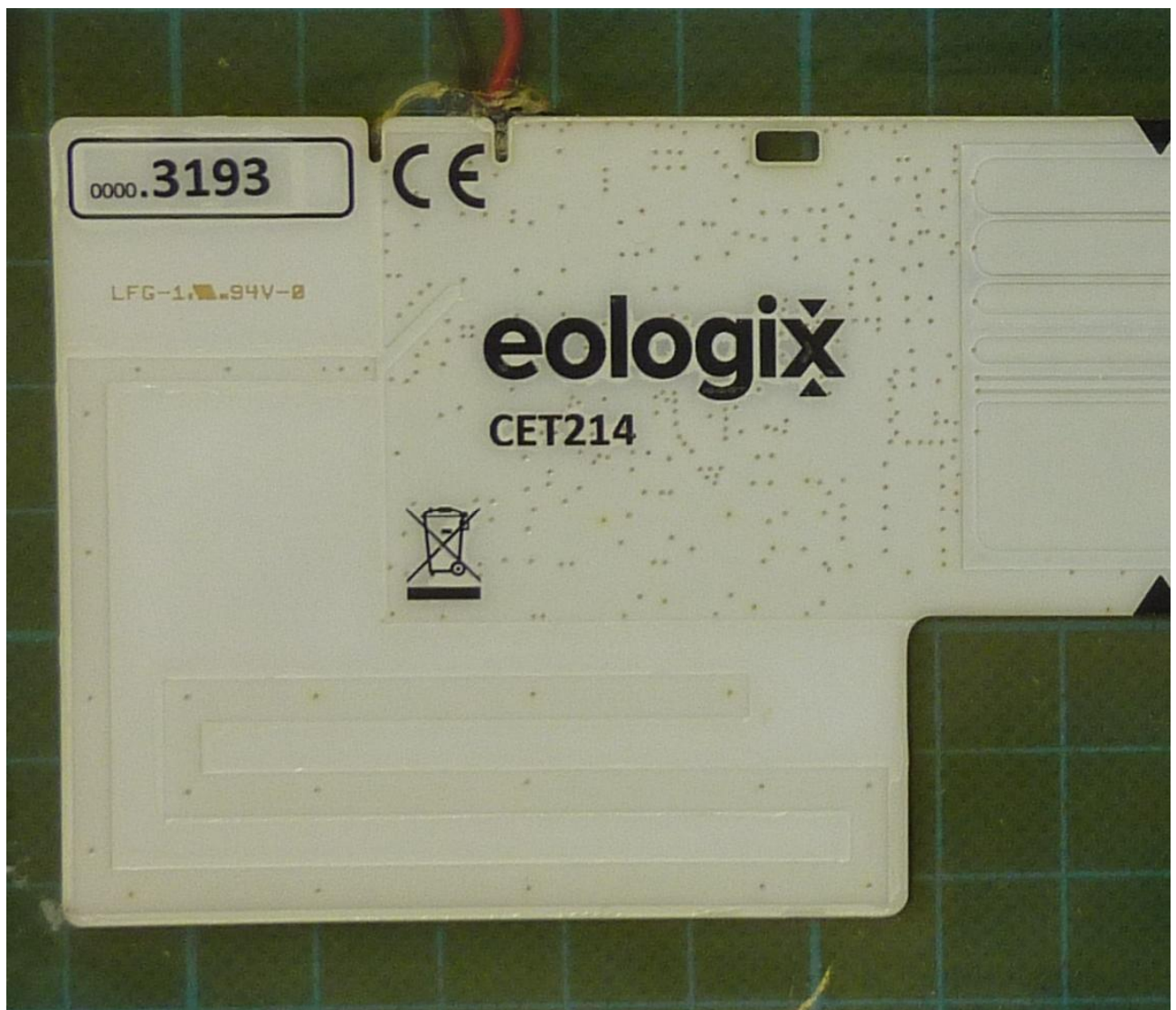
PCB – top view, transmitter and integrated antenna
