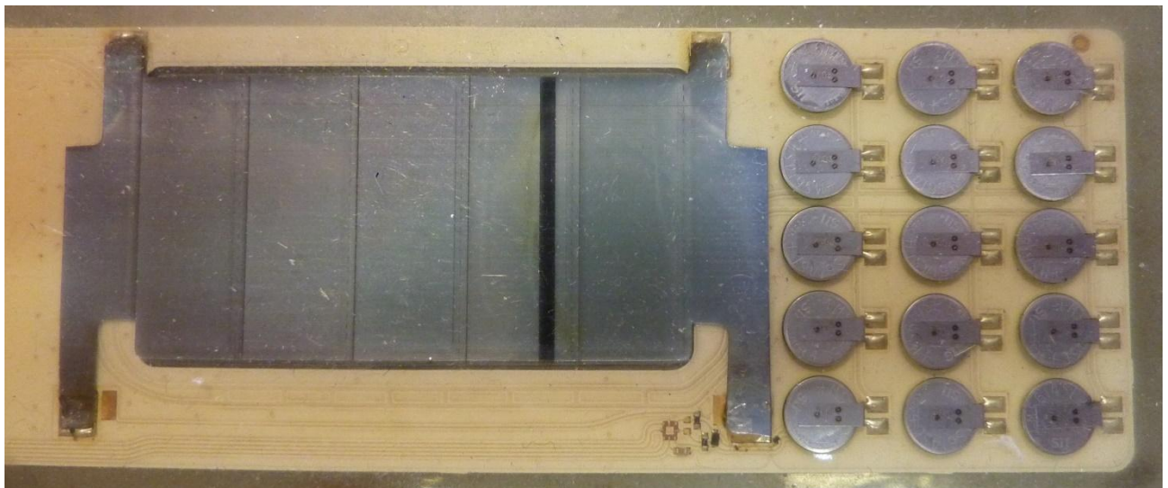
PCB – bottom view, photovoltaic module and accumulators
