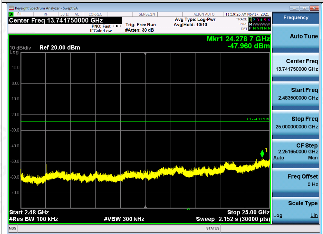
Test_Graph_802.11n40_ANT1_2422_MCS0_Higher Band Emissions
